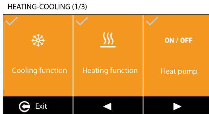
**HEAT PUMP Function** – Once the cooling function is activated in the Service Menu, the HEAT PUMP icon will appear, which corresponds to the connection with the external cooling unit – this icon must be activated.
