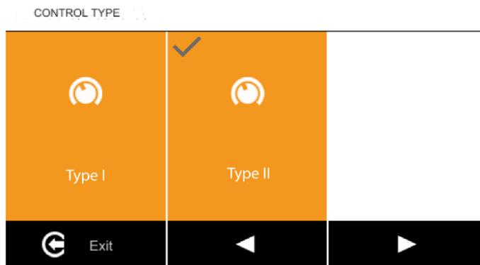
**TYPE I** – One output controls the activation and deactivation of the compressor, while the other output selects the heating or cooling mode.
