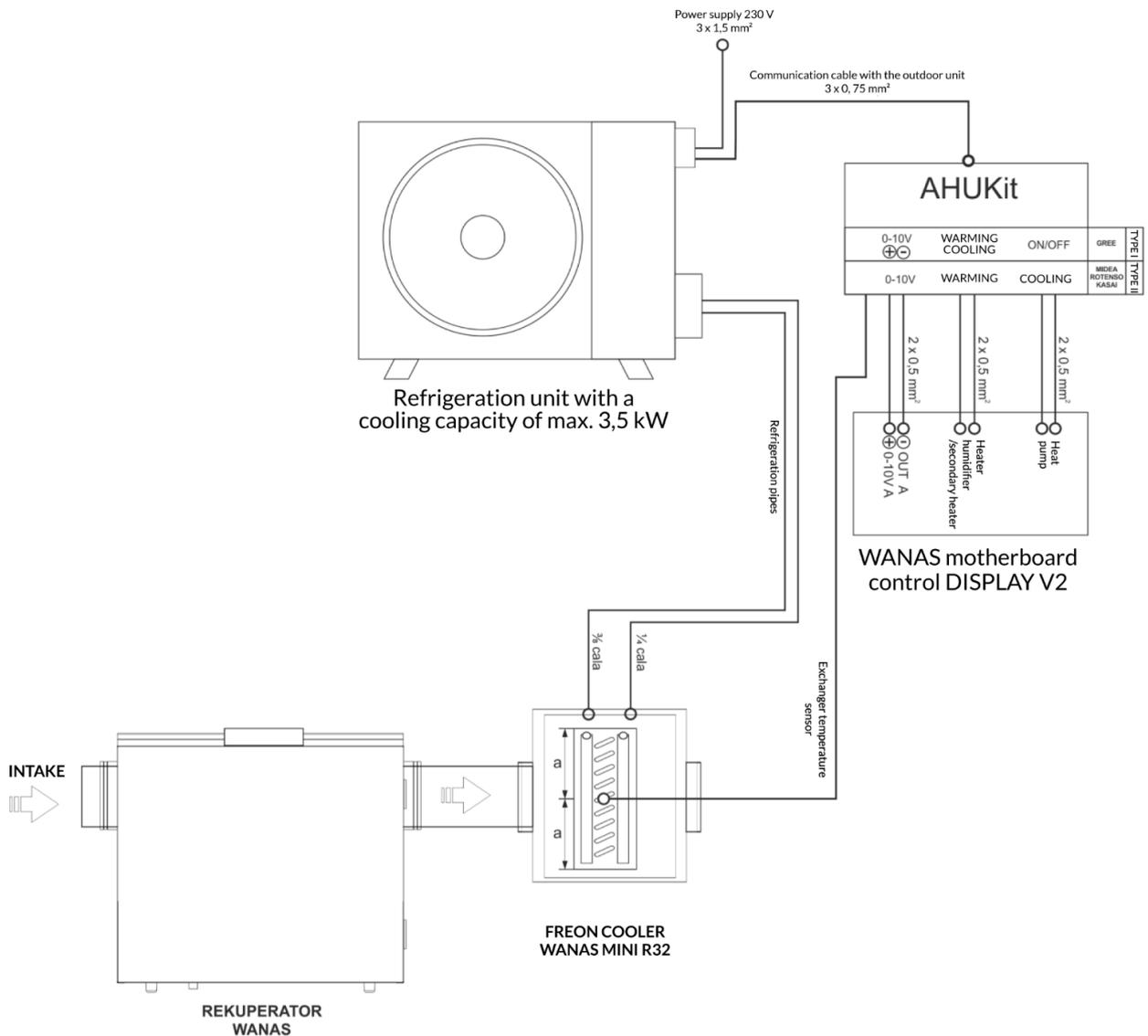
**WARNING:** After connecting the system, perform a leak test with nitrogen, followed by a leak test under vacuum – 0.5 bar. Fill the system with R32 refrigerant. If the distance from the external unit exceeds 5 meters, add refrigerant: 12g of refrigerant for each additional meter of installation. For distances below 5 meters, do not add refrigerant.
